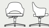
Conference Armchair - Relax Swivel 4 Star Base L 66.5 x D 64 x H 82/88.5 cm
